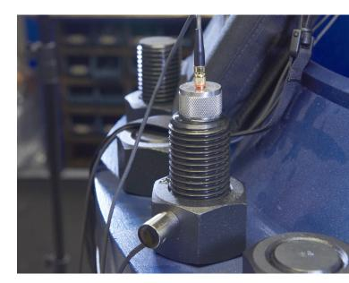
Measurement is achieved by determining the change in the transit time of an ultrasonic shock wave along the length of the fastener as it is tightened.
