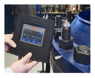
The Echometer Premier ultrasonic measurement device has been developed specifically for the bolting industry which measures, displays, stores and transfers bolt elongation and load. A hard wearing unit with a touch screen. The most advanced instrument available to control or verify bolt elongation and load in the field or laboratory developed with input from the most experienced users and electronic developers in the bolt tightening industry delivering a system with intuitive software.
