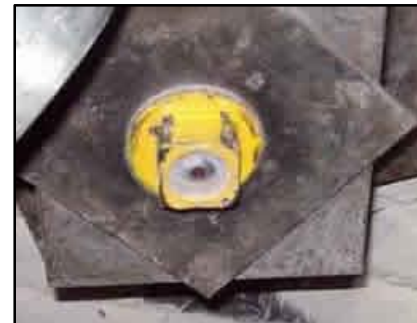
SmartBolt within designed tension limits
